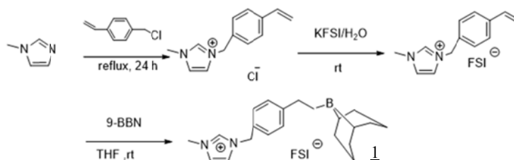
Fig 1. Synthetic scheme of novel organoboron molten salt
